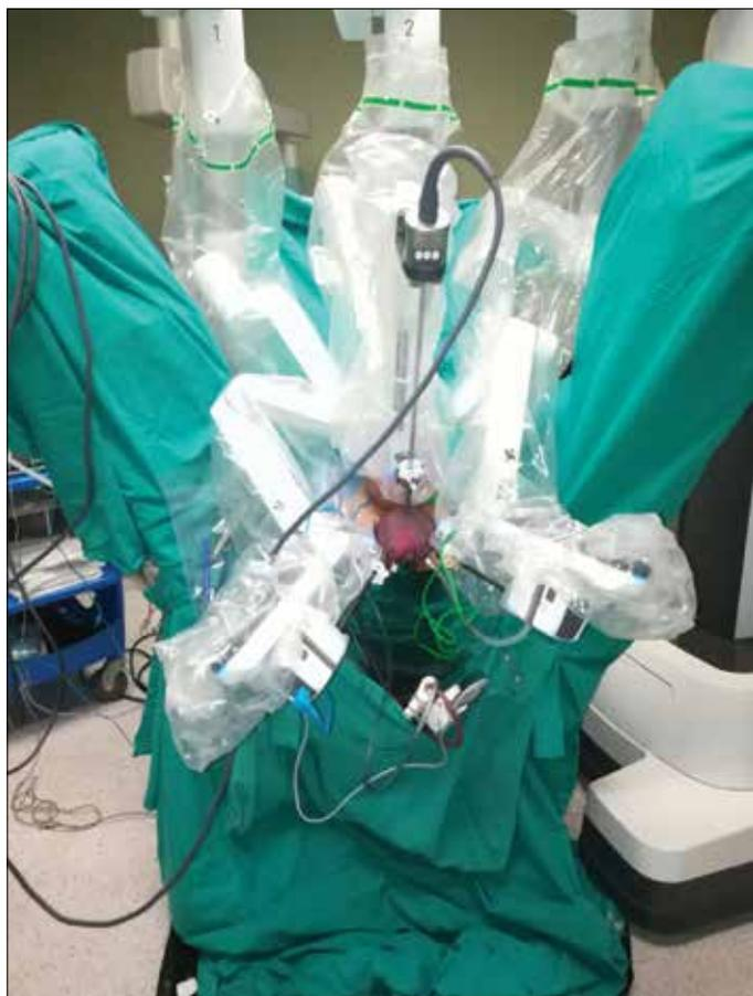
Figure 1. The docking of the three robotic arms
