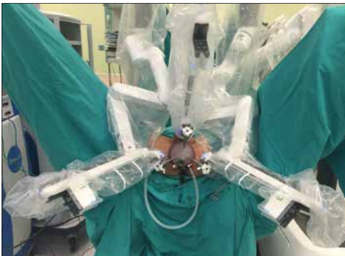
Figure 2. The docking of the three robotic arms
